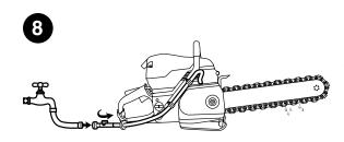
Attach to water source with pressure of not less than 20 psi (1.5 bar).
